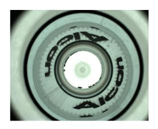
OCR inspection at the bottle neck. (This image need to unwrapped to proceed for OCR inspection)
