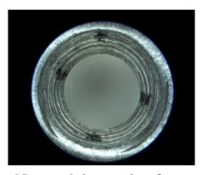
Nut track inspection for checking the black spot.
